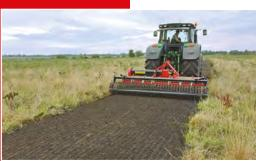
Built with a working width from 145 to 600 cm, required power from 100 to 360 HP and working depth from 15 to 38 cm. EXTREME stone burier can achieve a high quality result in extreme conditions without deforming the machine's frame.
