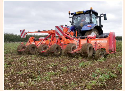
Foldable The 6/8-row haulm toppers can be hydraulically foldable as an option.
