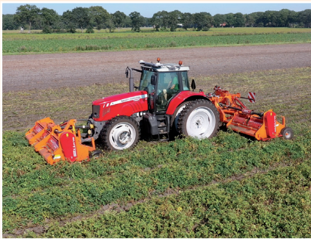
Triple Glutton With the optional 'Triple' version, the foldable Glutton is mounted behind the tractor and the 2- or 4-row Glutton is mounted at the front.
