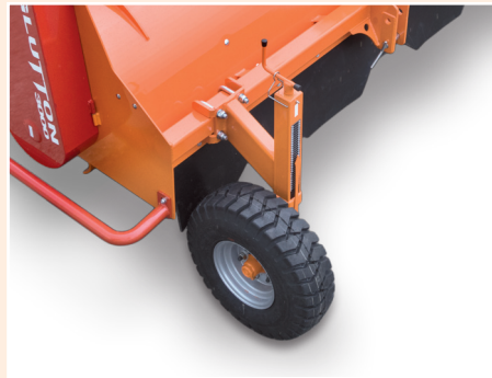
Tyres with spindle adjustment The topping height is set by depth adjustment wheels with spindle adjustment. Hydraulic adjustment of the depth adjustment wheels is optional.
