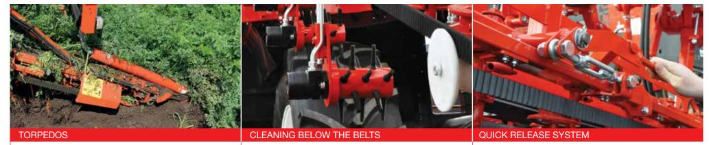
The 2 (optional hydraulically driven rotary) torpedos per element ensure an accurate intake of the haulm. If you want, as a driver, to concentrate better on the actual harvesting process, you can opt for DAS (Dewulf Automatic Steering). Two robust sensors detect the crop and correct the positions of the cylinder on the pole.
