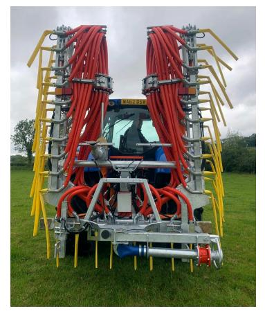
Twin Macerator Vertical Dribble Bar/Band Spreader (10m/12m/16m)
