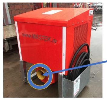
The PTO shaft must be connected to the front side of the compressor If being operated by the rear P.T.O. on the tractor
