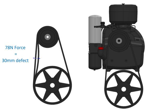
**NOTE:** If the belt squeaks when running, check the tension and adjust if necessary. If the noise continues, replace the belts.
