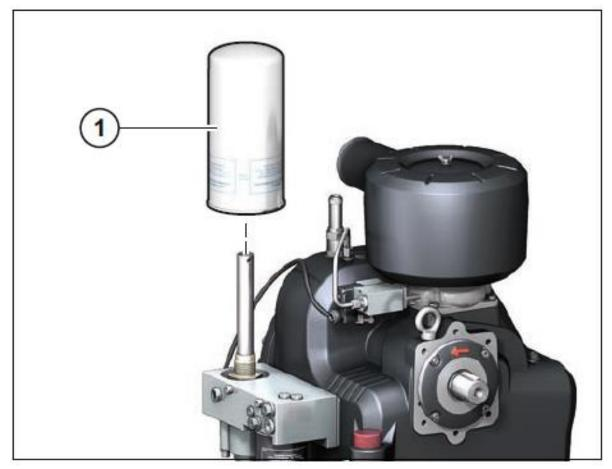
The separator cartridges must only be replaced when the compressor system is stopped and completely depressurized.
