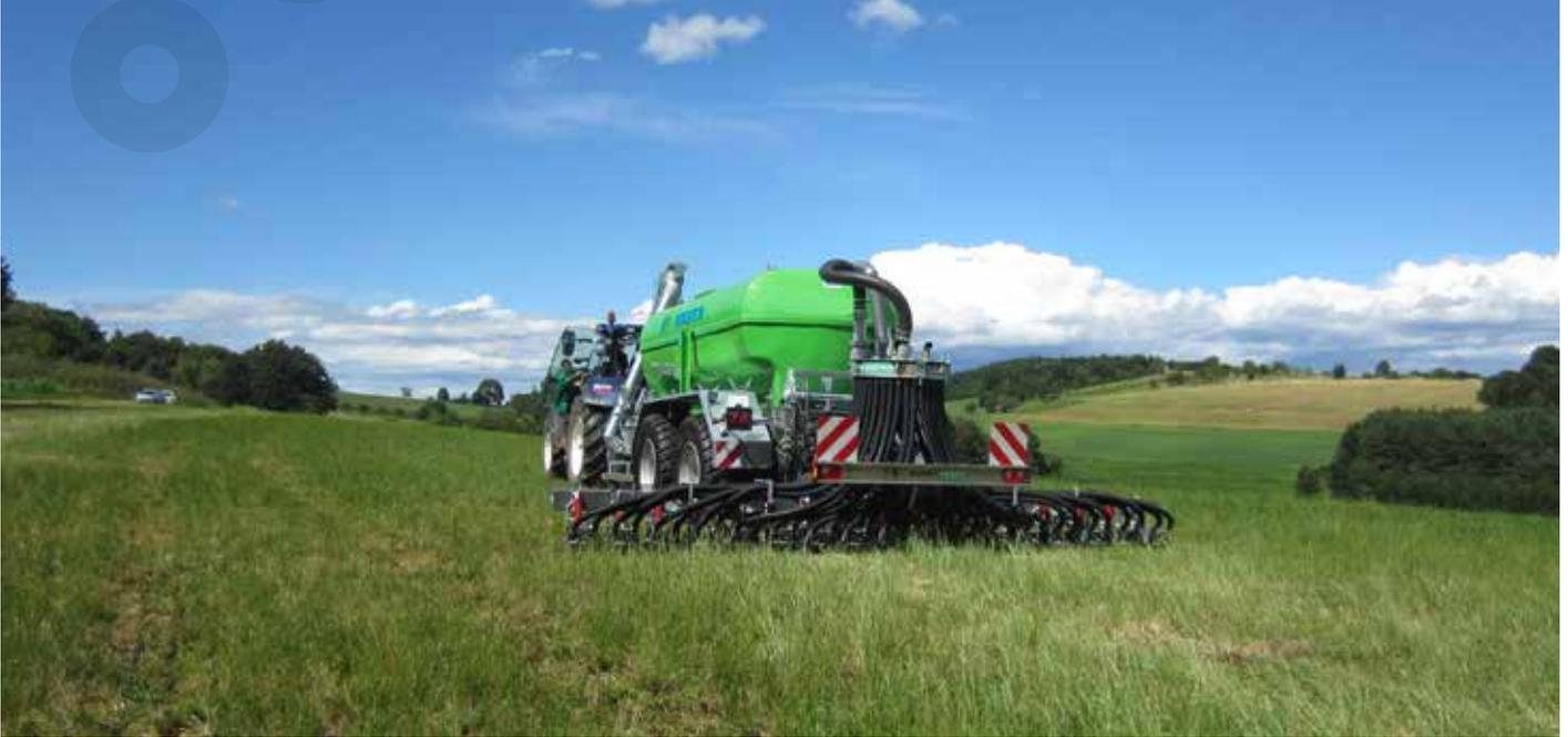
The lightweight disk injector is specially designed for attachment to slurry tankers to keep the empty weight of the slurry tanker as low as possible. The 50 mm wide flow hoses are evenly supplied by a central distribution head and deposit the slurry in slit rows 20 cm apart. The 305 mm, three-part disks open up 2-6 cm slits in the ground and are arranged in disk pairs. Each disk pair is equipped with caster steering and a mechanical drip stop.
