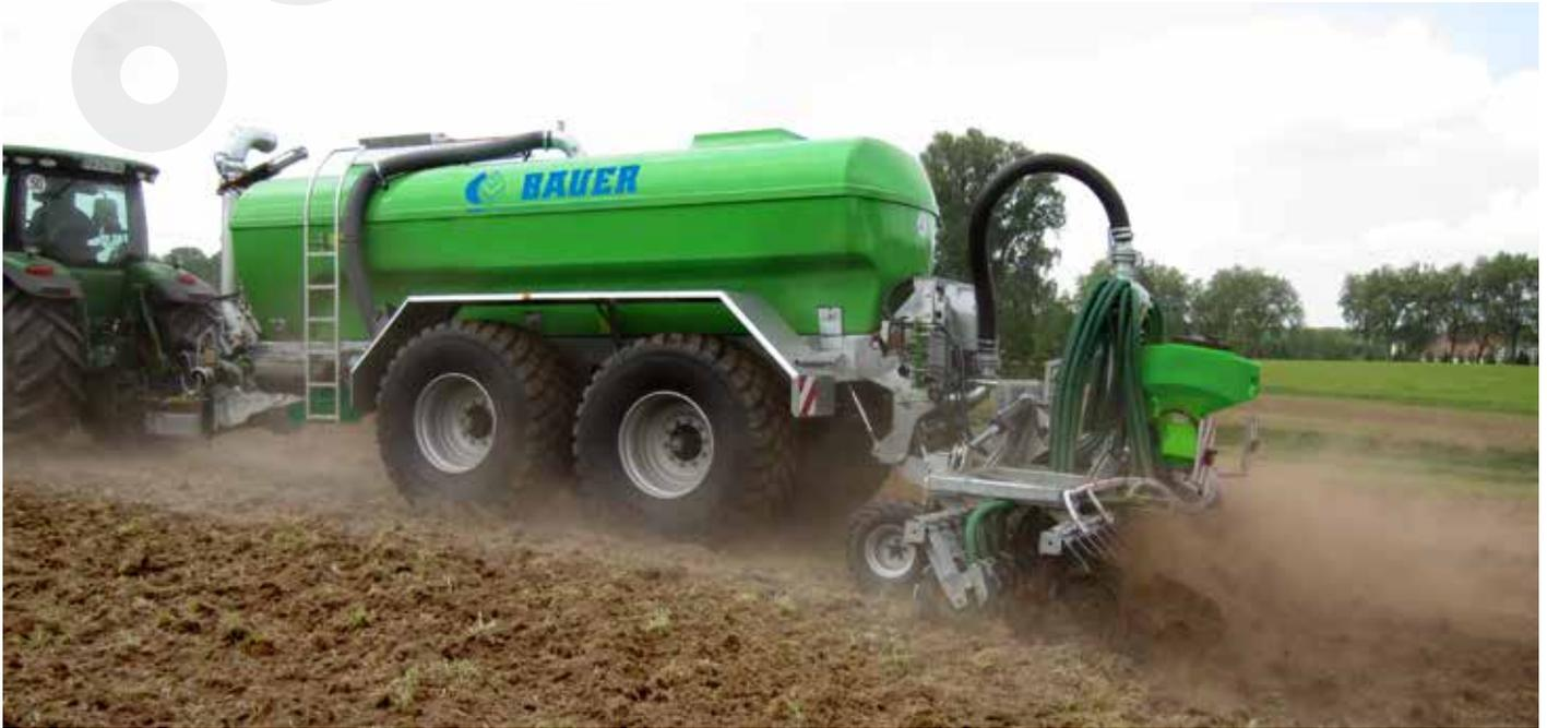
The Cerres S disk harrow works the slurry into the ground in a single step. The two rows of toothed disks introduce the slurry into the ground gently, in a flat profile. Maintenance-free bearings and a disk diameter of 510 mm make the Cerres S an economical machine that was designed specifically for attachment to slurry tankers.
