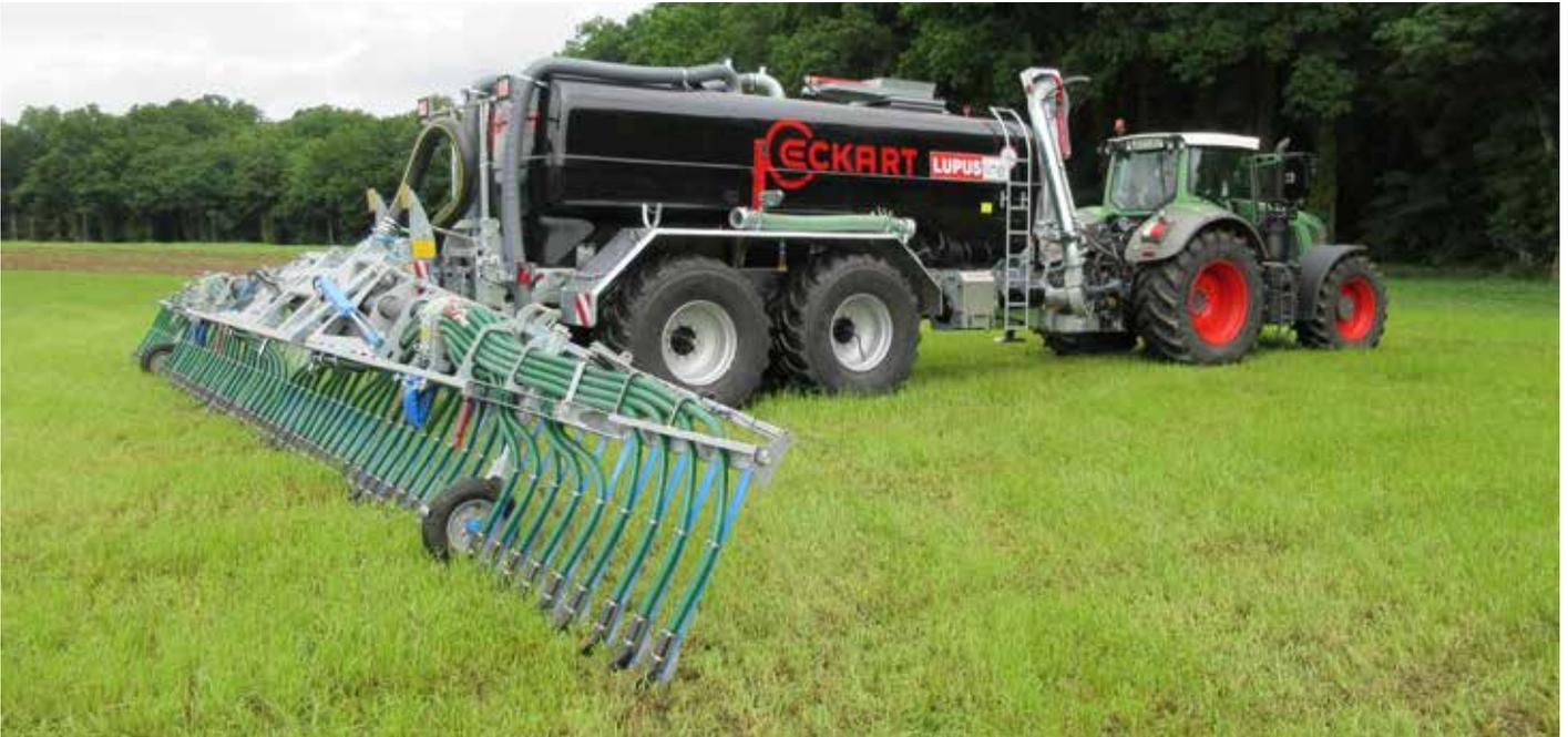
The drag shoe applicator has specially shaped drag shoes that open up the crops and deposit the slurry directly on the ground. The 40 mm wide flow hoses are evenly supplied via one or two Bomech distribution heads and positioned at 25 cm intervals. A slope compensation system optimally adapts the individually spring-loaded drag shoes to the terrain. Undesired dripping is prevented by swinging the flow hoses to an upward position.
