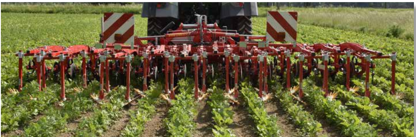
A preloaded spring ensures consistent working quality of the finger weeders
