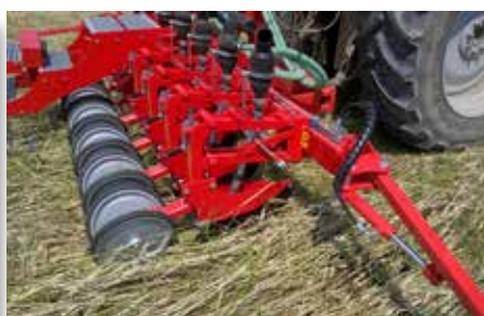
Operation of the CHOPSTAR-SEEDER in direct seeding
