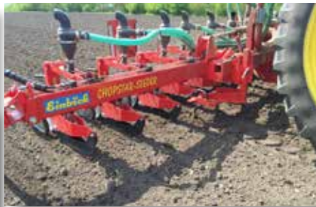
Seeding of soybeans with the CHOPSTAR-SEEDER.
